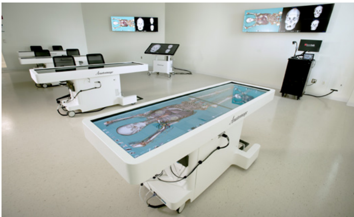
Within the Anamatage Lab, each table is capable of displaying horizontal slices of the human body to reveal bone structure, nerves, muscle, and veins without having to physically dissect a body. The NAV system enables content to be captured and distributed to remote locations over the university network.
